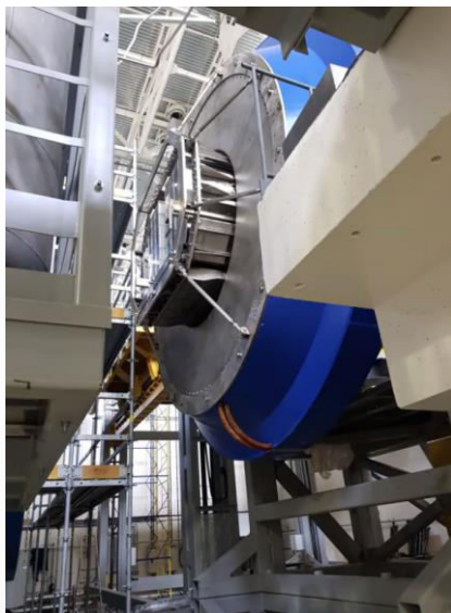
FHCAL assembled on the platform, ready to be installed in the Poles (modules are equipped with FEE)
