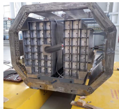
FHCAL assembled on the platform, ready to be installed in the Poles (modules are equipped with FEE)
