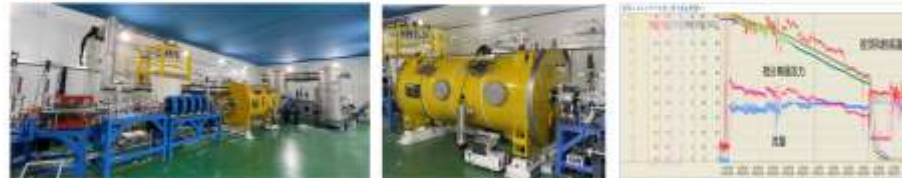
CEPC collider ring 650MHz 2-cell short test module has been completed in TDR phase
